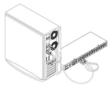
5. Locate your next input cable. Repeat step 2 with all the computers that will be attached to your master SwitchView OSD. Next, attach the remaining computers to the slave SwitchView OSD.
