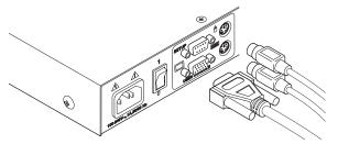
5. Locate the power cord that came with your SwitchView OSD unit. Plug it into the IEC power connector on the SwitchView OSD. Make sure that the SwitchView OSD power switch is off, then plug the other end of the power cord into an appropriate AC wall outlet. This outlet must be near the equipment and easily accessible to allow for unplugging prior to any servicing of the unit.
